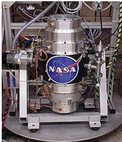
Figure 1: NASA G2 flywheel
